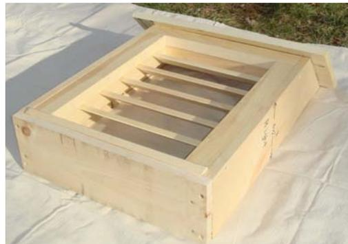
Fasten the top piece in the same manner. You'll notice that the top piece is over-sized. You will center this piece onto the bat house leaving an equal amount hanging off each side. When centered there should be a 2-inch overhang on each side of the bat house.
